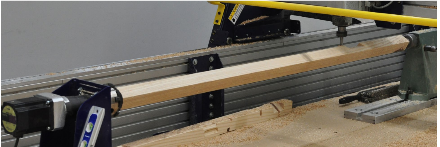
4-axis mill cuts joint pockets.
